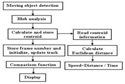
Fig.4: Algorithm for tracking and speed measurement
