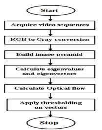
Fig.2:Agorithm of moving object detection
